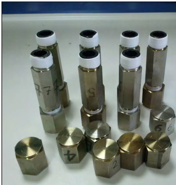
HTC autoclaves at TU Crete
